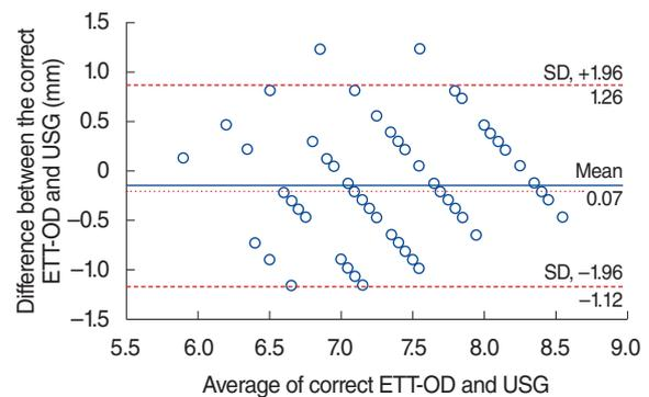
**Fig. 3.** Bland-Altman diagram showing the magnitude of the difference between the correct ETT-OD and USG (n=114; mean bias,  $0.07$  mm [solid line]; SD,  $0.61$  mm). The dashed lines represent the lower (LL) and upper limits (UL) of agreement: LL,  $-1.12$  mm; UL,  $1.26$  mm. ETT, endotracheal tube; OD, outer diameter; USG, ultrasonography; SD, standard deviation.
